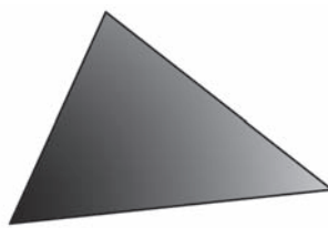
Figure 10.11. A Gouraud-shaded triangle with different shades of gray at the vertices.
