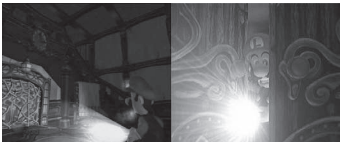
Figure 10.29. The flashlight in Luigi's Mansion is composed of numerous visual effects, including a cone of translucent geometry for the beam, a dynamic spot light to cast light into the scene, an emissive texture on the lens, and camera-facing cards for the lens flare.
